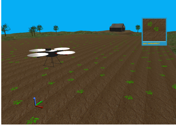
Figure 1: Platform simulation on MORSE. At the upper right corner, the UAV's semantic camera framing weeds.
