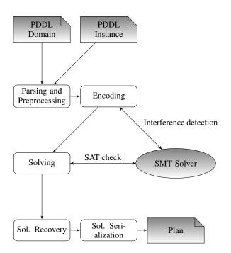
Figure 1: Basic architecture and solving process of the RANTANPLAN solver
