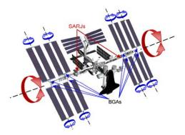
Figure 1: Solar arrays connected via rotary joints to ISS (taken from (Frank, 2012)).
